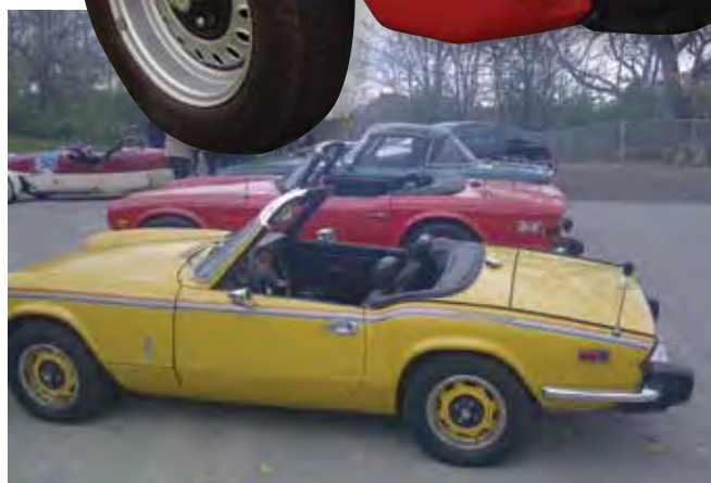
The North American Spitfire 1500 is easily identified by the big plastic over-riders and reflectors on the front and back wings
