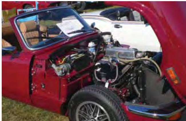
1974 Mk IV Spitfire - the forward hinging hood included the wheel arches giving full access to the engine and front suspension
