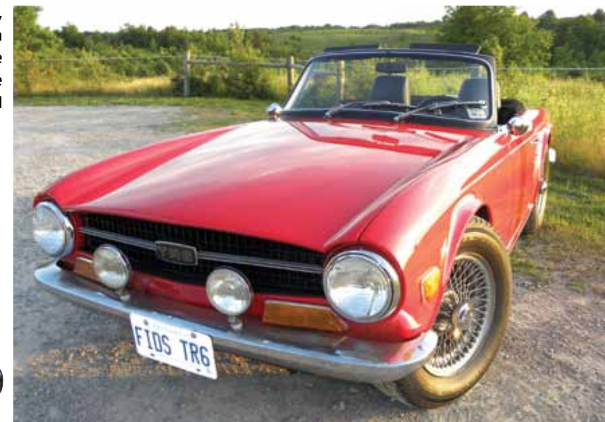
The front and rear panels, including the position of the headlights, were changed radically from the earlier TR5/250 model
