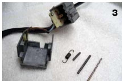
In photo 3, you can see the outer casing, the small spring and the two pins. By removing the shorter pin, it will allow you to slide the lever forward to expose the copper contacts. This is where you will be happy you're working over the towel, as there is a spring loaded ball and small insulator that may fall out of the lever head. I did not remove the
