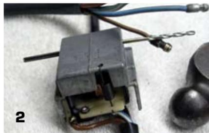
In photo 2, you will see that I used a 1/16" drill bit as a punch to remove the pin. There is also a second shorter pin that holds the lever to the casing and it is removed using the same method. The flash to pass contact tab needs to be bent slightly out of the way, to separate the casings. This will also expose it for cleaning later on.
