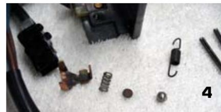
Photo 4 shows all the parts exposed. The goal is to clean all six circular copper contacts and the copper "shoe" that rides over four of them. To do this, I used a moist paste of "Bar Keepers Friend" on the end of a Q-tip swab and some very fine sandpaper.
