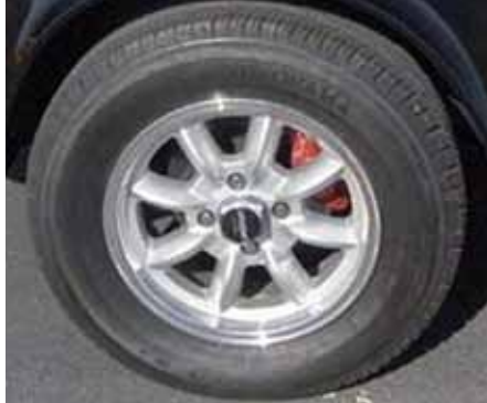
Panasport, Minilite or KN replicas make excellent replacements for TR6 or Spitfire wheel rims
