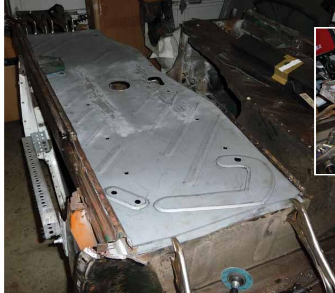
Floors are clamped into place before the outer sill is removed
