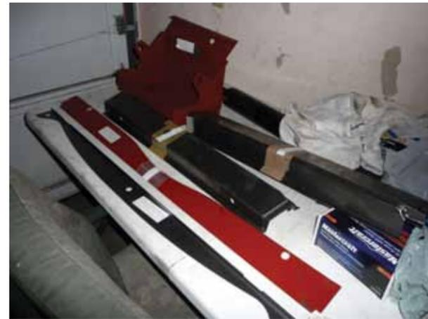
New metal pieces including the battery box, outer sills and bottom closing panels for the rear apron
