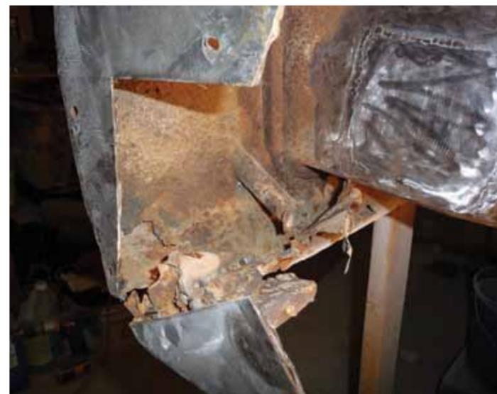
Rear passenger side fender/rear valence damage
